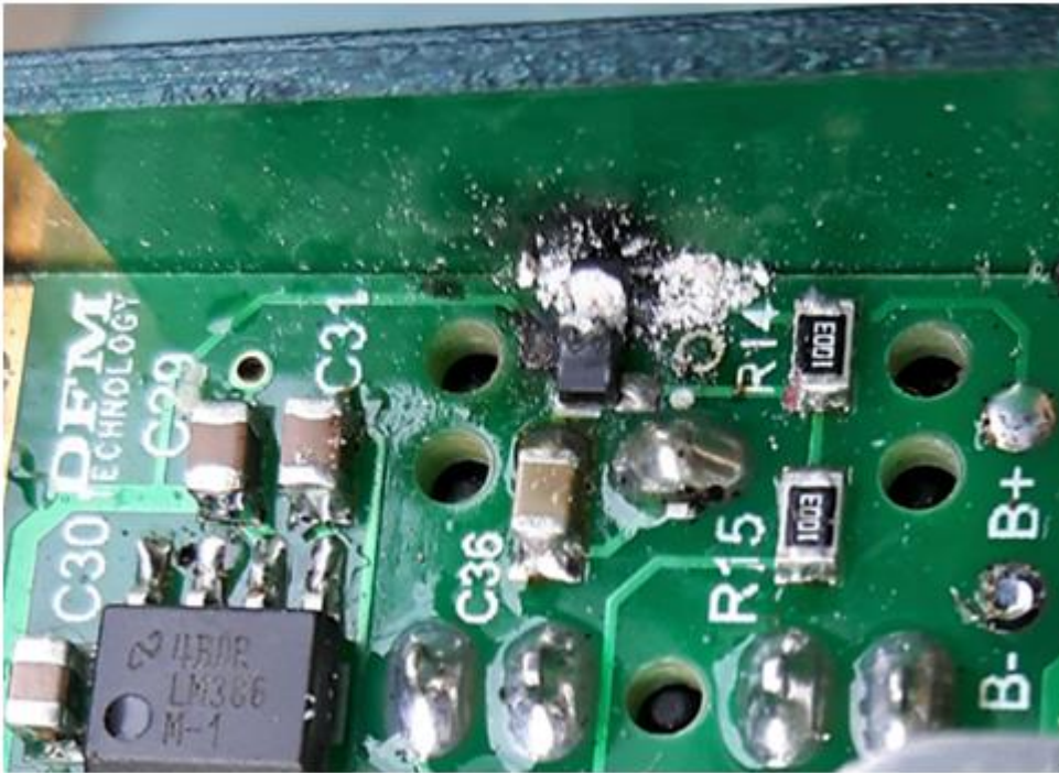
The above picture shows exploded MOSFET Q3. The voltage regulator U5 was also blown.
