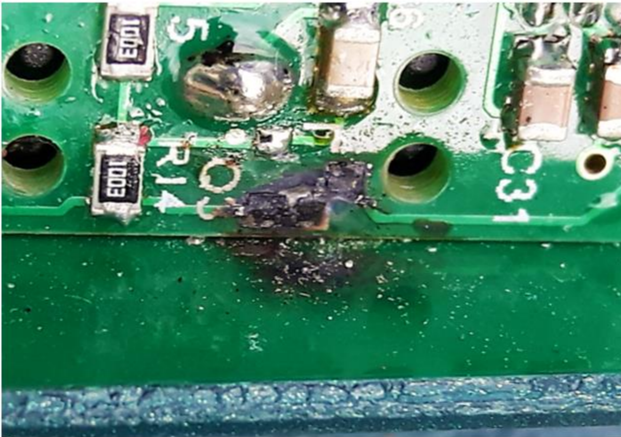
The above picture shows exploded MOSFET Q3. The voltage regulator U5 was also blown.
