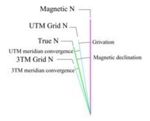
Magnetic N is the direction of the local magnetic field vector horizontal component.
