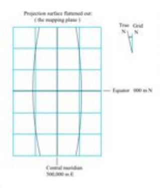
Meridian convergence (the angle of grid north relative to true north) is a function of both latitude and longitude.
